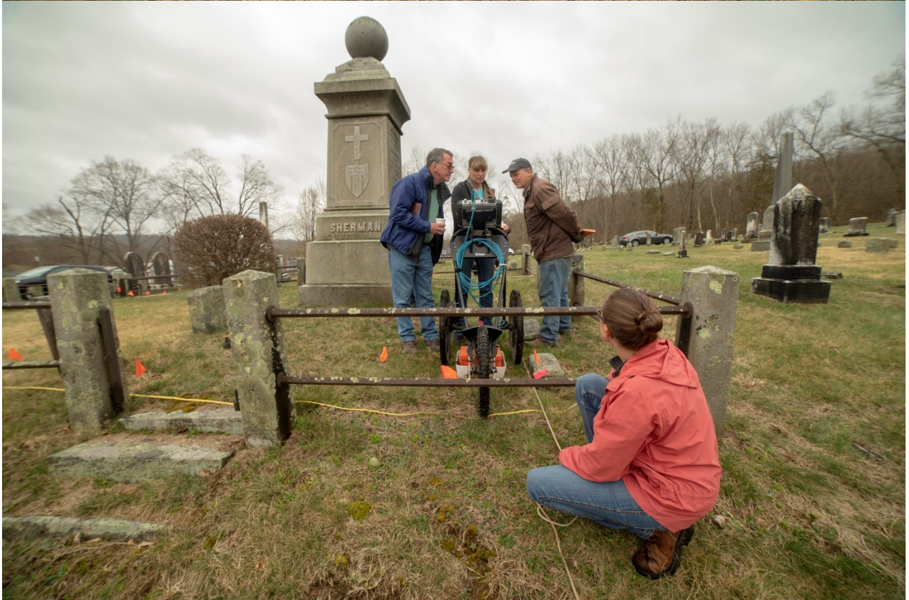
Figure 5. A GPR grid survey, conducted around the Sherman Family monument, was laid out using orange-colored flags (photo courtesy of Chris Randall).
